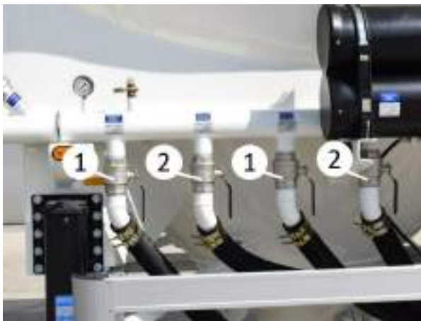
Jet air and fluidiser air connections
