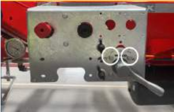
Fixing of suspension height
