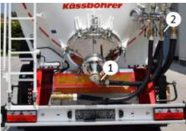
Fluidiser air line and valve
