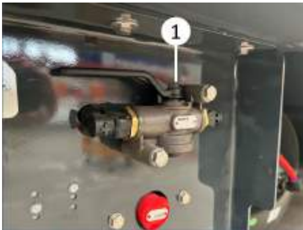
Self-steering axle release valve
