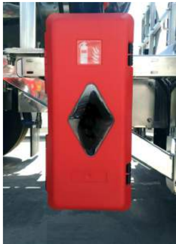
Fire Extinguisher Box
