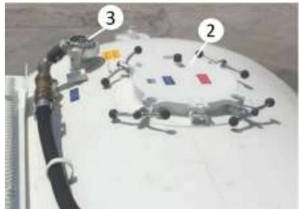
Filling manhole and filling neck
