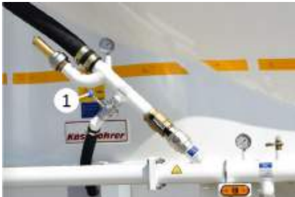
Air discharge valve
