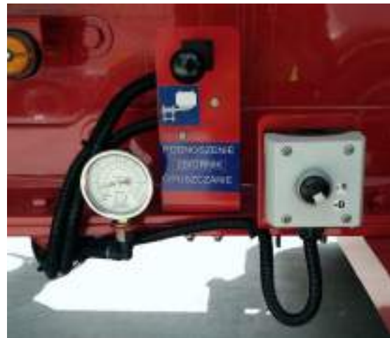
Hydraulic control panel
