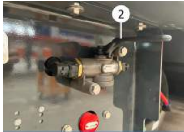
The self steering axles release valve
