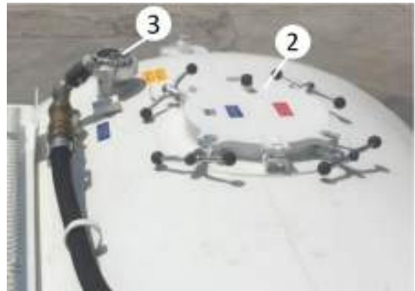
Filling manhole and filling neck
